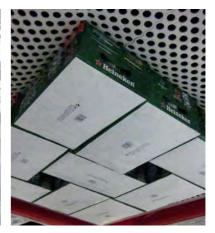
UniGripper LayerGrippers can be equipped with many accessories, such as hooks for pallet hand-ling, suction cups for lifting slip sheets and floating attachments for automatic alignment of the LayerGripper with the layer. The UniGripper LayerGripper is offered as a complete system including selected side channel blowers for vacuum generation and smart solutions for the installation of the vacuum hose.
