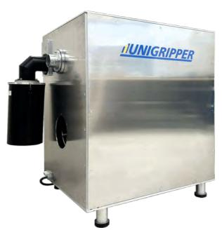
UniGripper Silent Power comes in two sizes, one size for vacuum flows up to approximately 1000m3/h and one for flows up to approximately 1500m3/h. UniGripper Silent Power reduces sound levels around 10-20 dB. From app. 80-90 dB without the silencer cabinet to app 65-75dB with the cabinet. Exact level that is reached depends on blower model and application.
