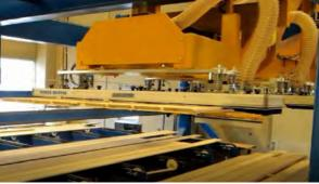
The UniGripper offering can include many or few of the components needed for such a vacuum handling system. Either only the grippers with the vacuum generation equipment — typically a side channel blower — to lifting frames two or more gripping units and distribution pipes for distributing the vacuum between the gripping units.
